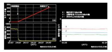
Initial magnetic field data obtained at mast deployment
