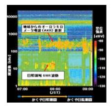
Electromagnetic environment observed by LRS wave receivers
