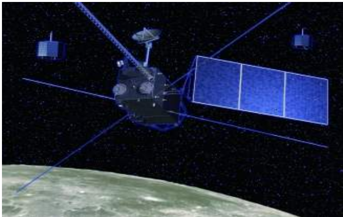
Gravity measurements by KAGUYA to give information on the shape of the Moon.
