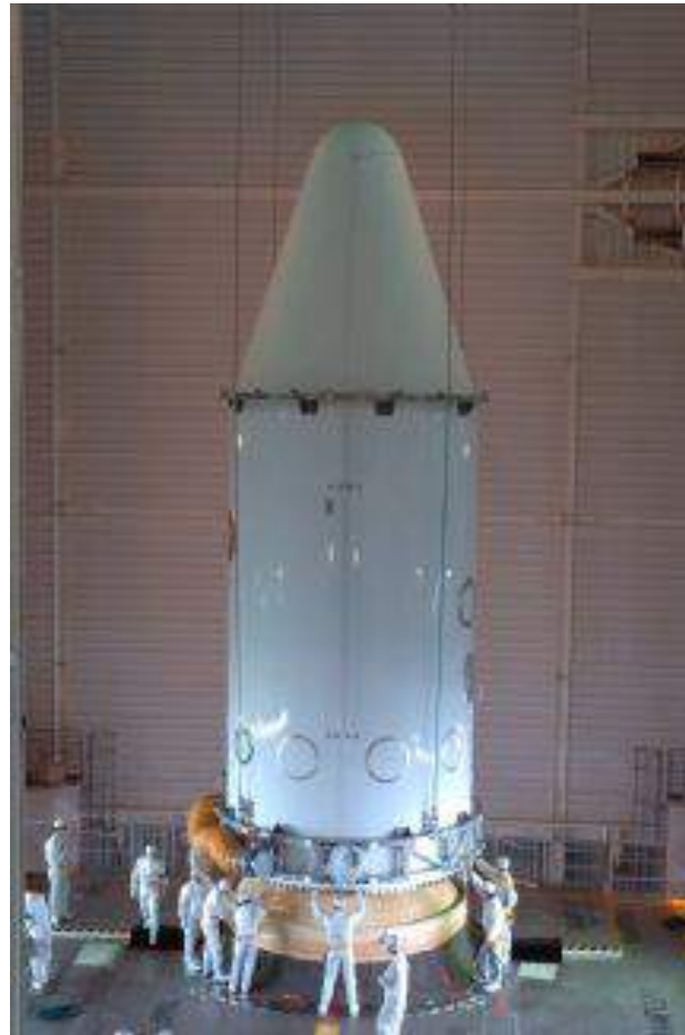
Integration into the nose fairing of H II rocket just before launch
