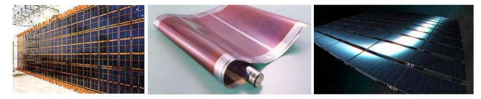
Conventional solar array panel for space use, with high performance cells, but heavy
