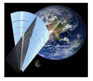
Basic Microwave-type Power generation/transmission panel suspended by wires Simple, but lower power efficiency (USEF/METI)
