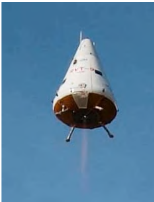
Reusable sounding rocket under development in JAXA. Vertical takeoff and landing.
