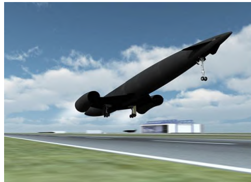
Reusable space plane, Skylon, using Synergistic Air-Breathing Rocket Engine, designed by British company REL.
