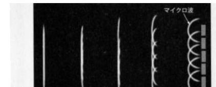
Electromagnetic wave radiated from an array of small antennas with a same phase
