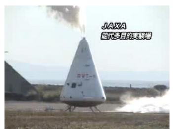
Small scale reusable rocket experiment in JAXA Weight : 500kg, Length: 3.5m
