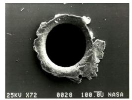
Damage in hypervelocity impact
