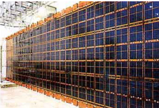
Conventional solar array panel for space use, with high performance cells, but heavy
