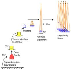
Fig.1 SSPS typical construction scenario.
