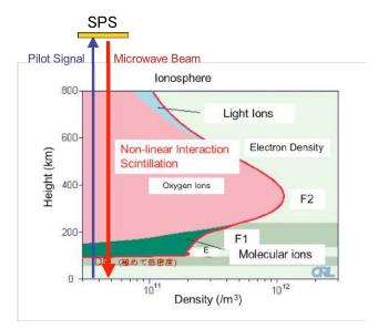
Fig.5 Possible interaction of strong microwave beam with the ionosphere.
