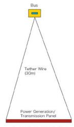
Gravity Gradient Stabilization
