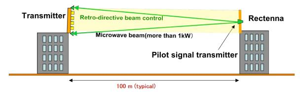
Fig.3 Configuration of the demonstration experiment.
