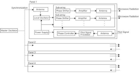
Fig.4 Block diagram of transmitting system.
