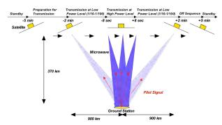
Fig.8 Experiment sequence in case of Mode A. The full power at 3.8 kW is transmitted to the ground for 16 sec guided by the pilot signal when the satellite is flying over the ground station.
