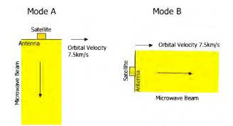
Fig.7 Two configurations of the demonstration experiment using the small satellite. The microwave beam is transmitted to the ground in mode A, while it is transmitted parallel to the orbiter velocity vector in mode B.
