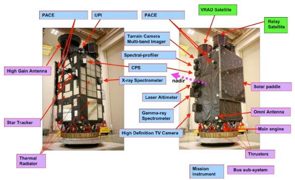
Fig.2 Configuration of bus subsystem and mission instruments.
