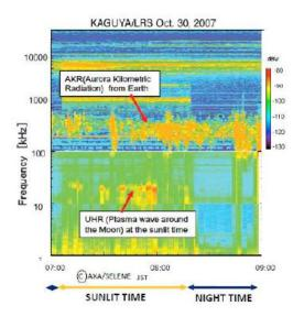
Fig.11 Wave spectrum observed by LRS wave receivers. Aurora Kilometric Radiation and UHR waves are detected.
